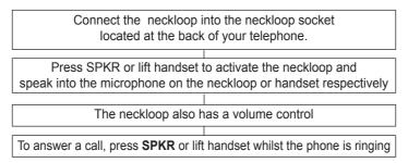
**Note**: The Ampli600 must be connected to the mains in order to use a neck loop.
