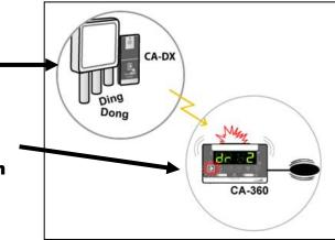
Install device on "existing door chime" or "intercom door announcer" for vibration detection.
