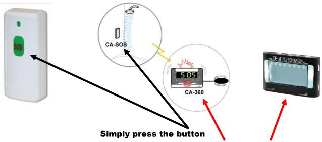
to send a wireless signal to activate Model CA-360 or CA-RX.
