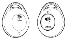
It takes up to 60 seconds to complete the registration. When the registration is successful, the red LED lights on the SOS pendant turns off, and the telephone base beeps and its visual ringer indicator light turns off.
